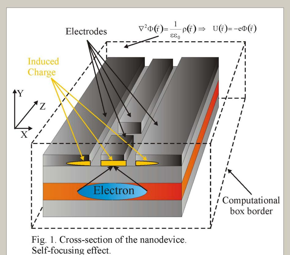
As the result of the self-focusing mechanism (caused by interaction with the induced charge) the electron shows properties unique for a quantum particle. It is able to tunnel through or reflect off a potential barrier with probability 100% (fig.2a, 2b). Such behaviour, characteristic for a classical object, is very rare for a quantum one, which usually partially tunnels through and partially reflects from the barrier (Fig. 2c).
