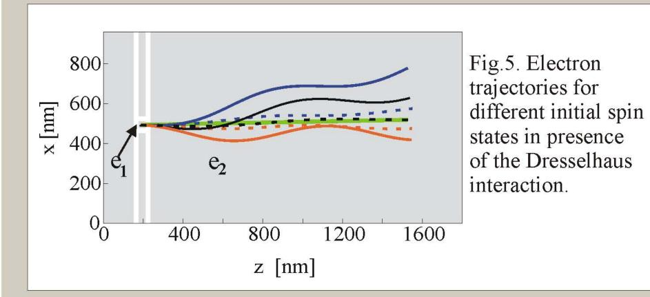
After setting in motion along the z axis, the electron with spin parallel or anti parallel to the movement direction goes straight. The trajectories in all other cases are curved lines.
