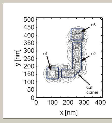
Fig. 3 Transport of the electron from under electrode e1 under e3 through e2. The cut corner of t e2 forces the electron to turn left.
