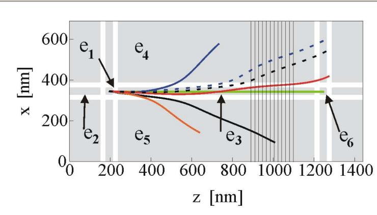
Fig. 6. The layout of electrodes in a nanodevice filtering-out electrons in spin state having any x or y component. The trajectories of electrons with different spins are marked as in Fig. 2. Spin up electron passes through the semimagnetic area (marked with vertical lines) and spin down electron reflects from it.
