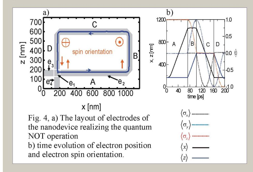
Applying adequate voltages on electrodes e1, e2, e3 and e4 it is possible to bind an electron under e1.
