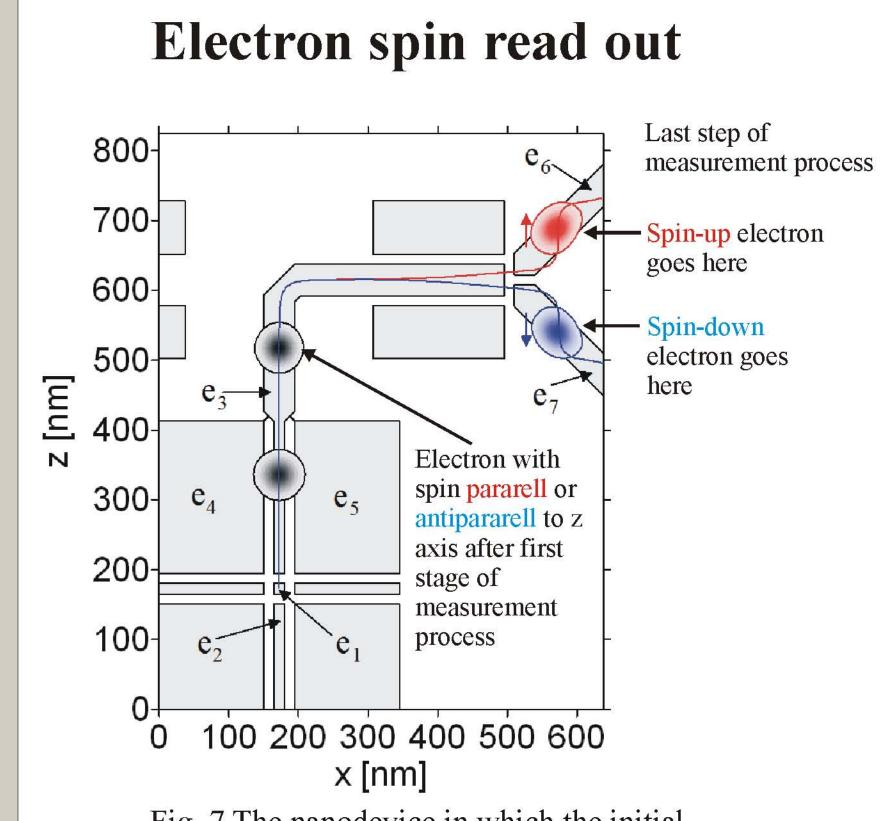
Fig. 7 The nanodevice in which the initial electron spin orientation is measured without applying external magnetic field.
