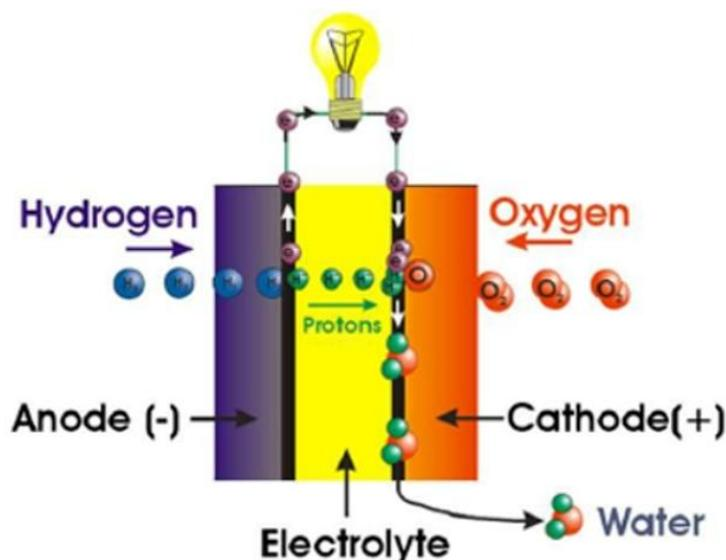
**Figure 1.6.** Scheme of proton-conducting hydrogen fuel cell and principle of its operation. Picture taken from [13].
