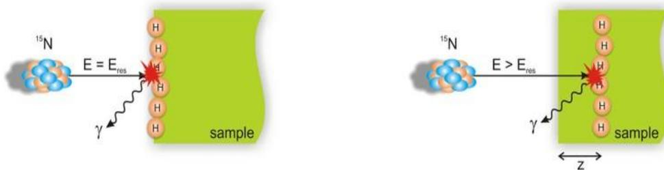
**Figure 2.23.** Principle of hydrogen profiling with the  $^{15}\text{N}$  method [135].
